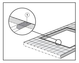
Grout lines ① and the hatched area underneath the surface of the appliance must be smooth and even. If they are not, the appliance will not sit flush with the worktop and the sealing strip underneath the top part of the appliance will not provide a good seal between the appliance and the worktop.
